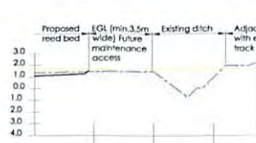
East Site Boundary Typical CS 6-6
